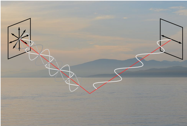
Fig. 2. Unpolarized sunlight is polarized by reflection off a smooth shiny surface. The direction of this polarization is parallel to the reflecting surface. In this case the horizontal surface of the water produces horizontally polarized light. "Figure 2" is a derivative of "Wire-grid-polarizer" ( https://en.wikipedia.org/wiki/Polarizer#/media/File:Wire-grid-polarizer.svg ) by Bob Mellish ( https://en.wikipedia.org/wiki/User:DrBob ), used under CC BY-SA 3.0 ( http://creativecommons.org/licenses/by-sa/3.0/ ). "Polarization by Reflection" is licensed under CC BY-SA 3.0 by Adam Blake.
