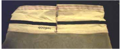
Figure 11. Net bag, showing Velcro strips sewn around edges
