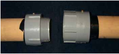
Figure 4. 3/4 inch Electrical conduit connectors shown in place on net handle.
