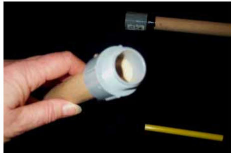
Figure 6. Net handle section, showing drill hole in centre of connector.
