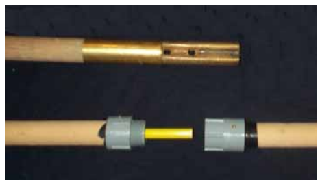
Figure 8. Close-up view of commercially available net-handle and brass fitting, shown with screw-together net section.
